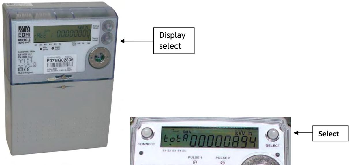
On the front of the meter there is a button called either SELECT or DISPLAY SELECT. When you press this button the screen should show the TIME. Further presses of the button will advance to other screens such as DATE and LAG. Pressing and **holding** the button for approximately 2 seconds toggles the screen between Set A and Set B. You should make sure that you are in Set A.
