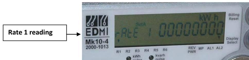
When you are on the last Rate, press the Display Select button a further 4 times and you should see the Total reading.
